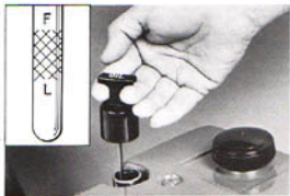
(Photo 26) Remove 8HP Kohler engine dipstick.
