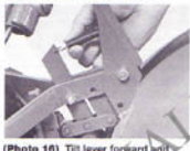
(Photo 16) Tilt lever forward and attach hook through tall vertical link.
