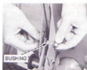
(Photo 14) Insert bushing and install bolt through upper hole in lever and yoke plates. Loosely add star washer and hex nut.
