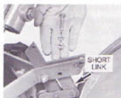
(Photo 13) Remove hardware that secures short link to yoke plates.
