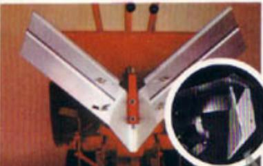
**HILLER/FURROWER:** The Hiller/Furrower hills corn, potatoes, etc. and helps to kill weeds in rows and between plants as it hills. Remove Hiller wings [no tools needed] and use Furrower alone to dig trenches for irrigation, drainage or trench composting (bulky organic matter and kitchen leftover for improving soil). Makes furrows to plant potatoes, corn, asparagus, etc. Furrows to 8" deep, hills to 8" high.
