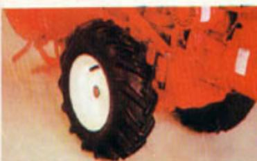
**BAR TREAD TIRES AND RIMS:** Especially helpful when extra traction is needed in loose, light, and sandy soils. Good for use with dozer blade, too. You can have your tiller equipped with these bar tread tubeless tires and rims (which most farm tractors also have). In place of diamond tread tires which are standard equipment.
