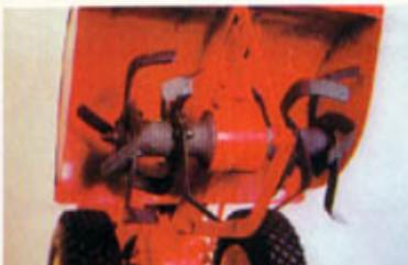
**BOLO TINES:** These are truly the all purpose Tines and are the type furnished on all new Troy-Bilt as standard equipment. For tilling in sod, weeds, cover crops, composted material as well as for seedbed preparation, tilling and cultivating. Their sweep-back "bolo" design sheds excess matter and prevents most tangling of roots, grass and vines. Unlike many other tillers, each individual tine is replaceable. Bolos till 6-8 inches deep. #01 Standard equipment on Horse and Pony models.
