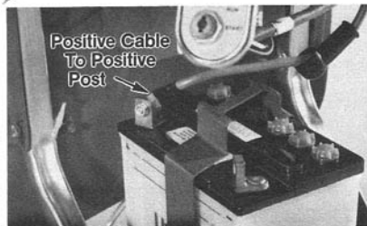
(Photo 2-11) On the 8HP electrical system, connect the positive (+) cable to the positive battery post as shown above. Use one of the small bolts and hex nuts to make the connection.
