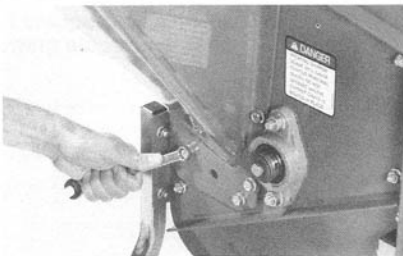
(Photo 2-5) Attach chipper chute to the side of your equipment. (8HP Model shown.)
