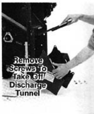
(Photo 5-19) Remove discharge tunnel.
