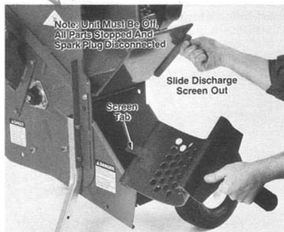
(Photo 3-8) Carefully slide the screen out. Note that there is a positioning tab at the far end of the screen. When installing the screen, the tab must go into a slot on the other side of the mainframe. Go to the other side of your machine and you'll see the tab protruding through the slot when the Discharge Screen is properly positioned. Remember to put all three rods back in and to secure them with the hairpins.
