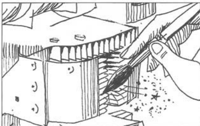
(Figure 5-5) Keep the engine cooling fins clean to prevent a potential fire hazard.
