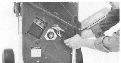
(Photo 5-26) Use 5/32" hex key wrench and a 1/2" open end wrench to take off hardware securing the chipper blade to the chipper flywheel. (5HP Model shown.)
