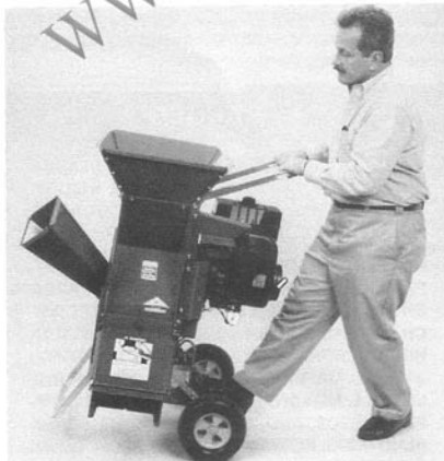
(Photo 4-1) To move your Chipper/Shredder, plant one foot on the axle, tilt equipment back with both hands until "balance point" is reached, then push or pull your equipment to a work area. Engine must be OFF.
