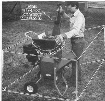
(Photo 4-4) When using the Shredder, stand 1-to-2 feet away from the top-loading hopper and release materials into it from any position within the "Operation Zone". (SHP Model shown.)
