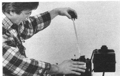
(Photo 2-7) On 5 HP Tecumseh engines, remove oil dipstick from oil fill tube, then add 19 ounces of motor oil using a clean funnel. Fill to "Full" mark on the dipstick. Do not overfill!
