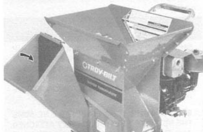
(Photo 3-3) The Chipper Chute is for processing larger, heavier branches. (8HP Model shown)
