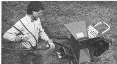
(Photo 4-2) Feed material into chipper at proper angle, and rotate branch. Do not overload the chipper. (5HP Model shown.)
