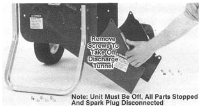
Note: Unit Must Be Off, All Parts Stopped And Spark Plug Disconnected
