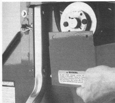
(Photo 5-9) Remove the belt cover held in place by two bolts and locknuts. The lower pulley and drive belt are behind it.
