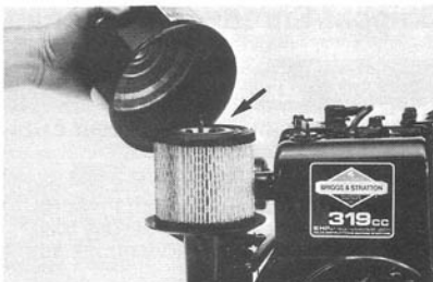
(Photo 5-3) Briggs & Stratton 8HP single-element paper cartridge air filter. (The 8HP I/C engine has a dual-element design — an outer foam filter and an inner paper cartridge.)
