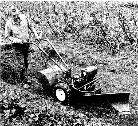
Using Dozer Blade for light grading.
