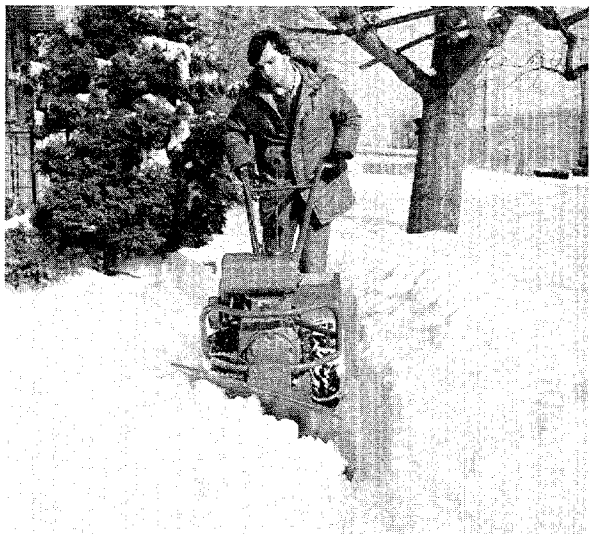
Clearing away snowfall with Dozer Blade.
