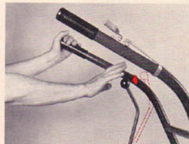
(Photo 2/11) When let go in Reverse, lever returns to Neutral.
