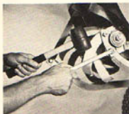
(Photo 8/64B) First, oil tight nuts.
