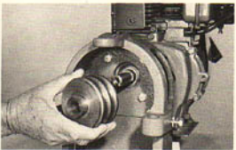
(Photo 7/38) Replacing the engine pulley.
