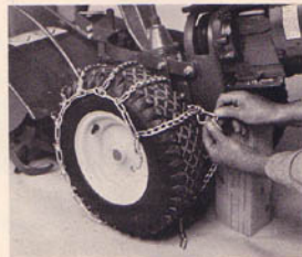
(Photo 6/9) First fasten chains loosely.
