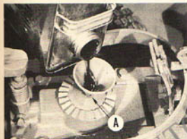
(Photo 1/7) Remove the T-bar and pour gear oil into transmission through hole at (A) handlebar base. It will take about 6½ pints (that's 3 quarts plus ½ pint). See photo. Use a funnel with a ½" tip to assist you.
