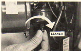
(Photo 7/52) Turn clockwise to lean fuel mixture.
