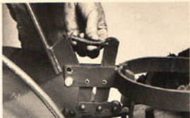
(Photo 8/148) Rehook lever and spring.
