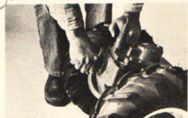
(Photo 8/30) Check for play in drive shaft.
