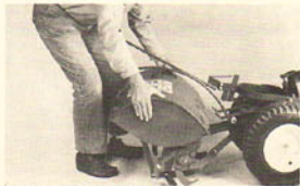
(Photo 8/43) Lift hood off.
