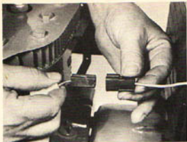
(Photo 8/92) Disconnect recharging wire.
