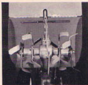
(Photo 5/8) BOLO TINES —The best general purpose tines for all soil conditions. Best for tilling under cover crops.
