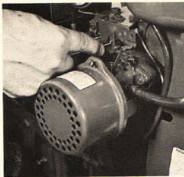
(Photo 7/43) Connect wire to speed control lever.
