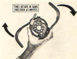
(Photo 8/72) Cutting edge of these hits soil
