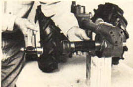
(Photo 8/21) Replacing seal with cover on.
