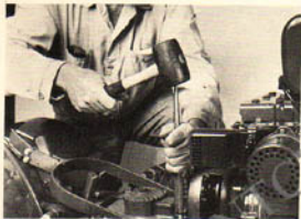
(Photo 8/109) Tap bars in place.
