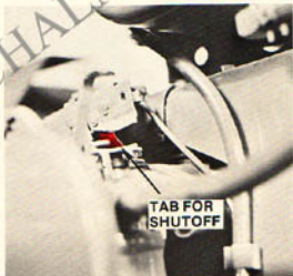
(Photo 7/45) Throttle control touches tab.
