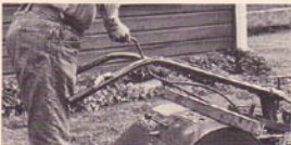
(Photo 6/22) If needed, bend lever.
