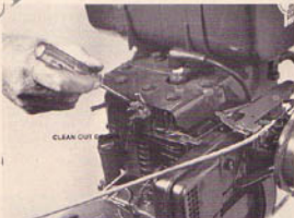
(Photo 4/2) Clean cooling fins.
