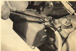
(Photo 8/133) Remove starter cable.
