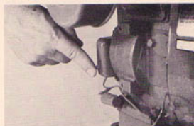
(Photo 4/32) Push in on stop button and hold it in, to stop engine.
