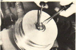
(Photo 8/26) Remove front snap ring.
