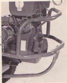
(Photo 6/31) Protects the recoil starter.
