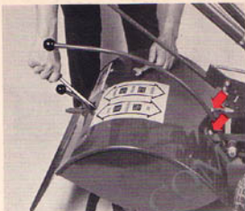
(Photo 7/7) Tighten bolts on head brackets.
