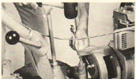
(Photo 7/33) Loosening upper pulley bolt.
