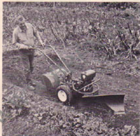
(Photo 6/16) Angle blade to one side to put soil where you want it.
