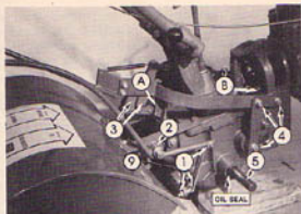
(Photo 7/2) Close-up of lubrication points.
