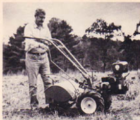
(Photo 4/22) Use Forward/Reverse lever to stop.
