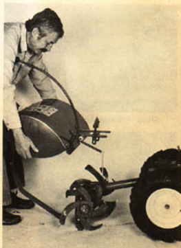
(Photo 8/140) Replace hood, lever and regulator
