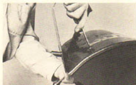
(Photo 8/41) Four rear hood bracket bolts.
