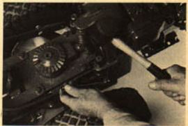
(Photo 8/147) Hold pressure on bolt and tap.
