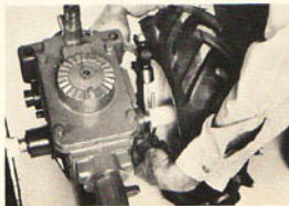
(Photo 8/3) Align holes with hex wrench.
