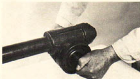
(Photo 8/22) Turn shaft forward and backward.
