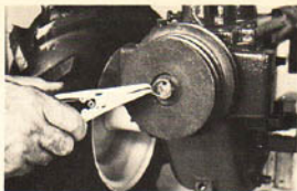
(Photo 8/24) Removing snap ring on lower pulley.
