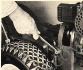
(Photo 8/98) Yoke is bolted to engine mount.
