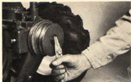
(Photo 8/120) Remove snap ring with pliers.
