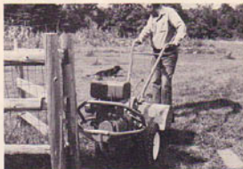
(Photo 6/28) Protects carburetor from fences, trees and doorways
