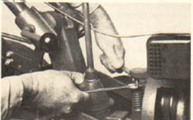
(Photo 7/29) Loosen locknut on adjustment bolt.
