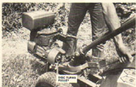
(Photo 7/27) Hold clutch lever in reverse.
