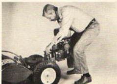
(Photo 8/107) Line up holes, put in bar.
