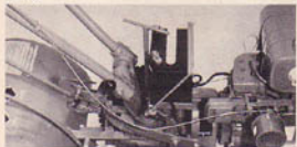
(Photo 4/10) Run throttle cable on electric start tillers down handlebars, as shown. Keep the throttle cable away from battery—6 HP electric start engine.
