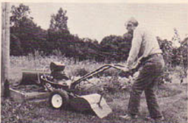
(Photo 6/23) Tine removal permits you to raise the front higher, and the blade banks easier.
