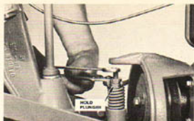
(Photo 7/30) If plunger turns, hold with pliers.
