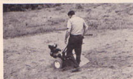
(Photo 5/14) Vertical Tilling on Slope—Tilling downhill and burying sod in one easy step.
