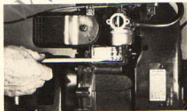
(Photo 7/57) Pencil points to drain hole.
