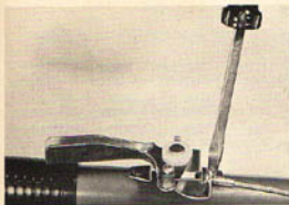
(Photo 1/15) Attaching the throttle control lever.
