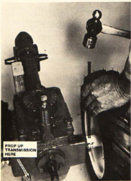
(Photo 8/129) Roll pin holds wheel on.
