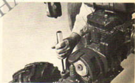
(Photo 8/118) Drive bar down and out.
