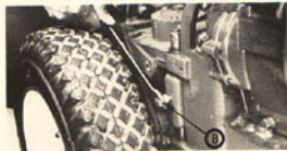
(Photo 7/34) Back off motor mount bar bolt B.
