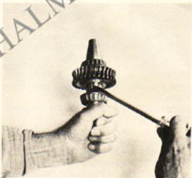
(Photo 8/15) Check key that drives bronze gear.
