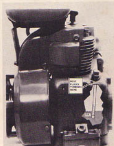
(Photo 4/26) 7 HP engine, rest dipstick's threads on top of hole. Don't thread in.
