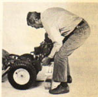
(Photo 8/119) Put engine on box.
