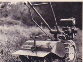
(Photo 6/44) In tackling tough sod, furrower can hold tiller back to allow tines more time to dig (use chains for traction).
