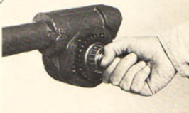
(Photo 8/18) Replace tiller shaft.
