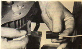
(Photo 8/132) Disconnect recharging line.
