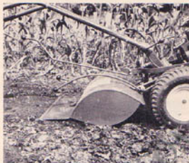
(Photo 5/19) Hood aids in pulverizing.
