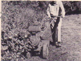
(Photo 2/10) To save your hands from being scratched by thorny bushes while tilling close to them, just move the handlebars to one side.
