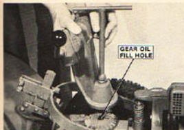
(Photo 1/7A) Remove T-bar to fill gear oil.
