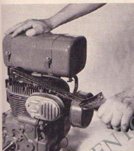
(Photo 4/41) Tightening head bolts on 7HP Kohler with a torque wrench.
