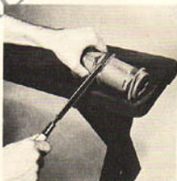
(Photo 8/62) File rough spots in groove.
