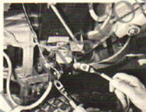
(Photo 7/59) Touch jumper to right post.
