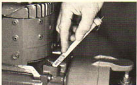
(Photo 7/55) Check oil level on 6 HP engines.
