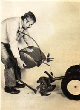
(Photo 8/126) Hood, lever & regulator come off.
