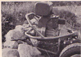
(Photo 6/30) Solid obstacles like stone walls won't damage recoil starter.
