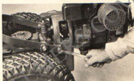
(Photo 8/149) Bolt yoke to motor mount.
