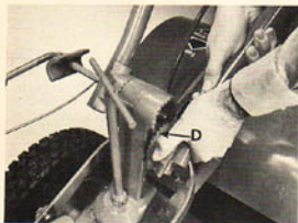
(Photo 1/13) Now force the handlebars apart and install the left inside ratchet, D .
