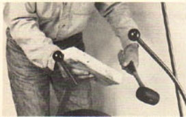
(Photo 8/42) Tap knob off, save tolerance ring.
