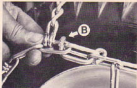
(Photo 6/10) Fasten chain tightly (tiller side).
