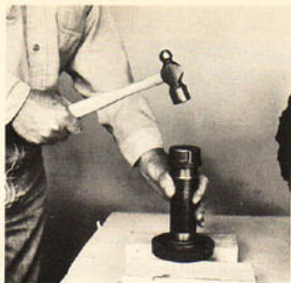
(Photo 8/12) Carefully tap seal out of cover.
