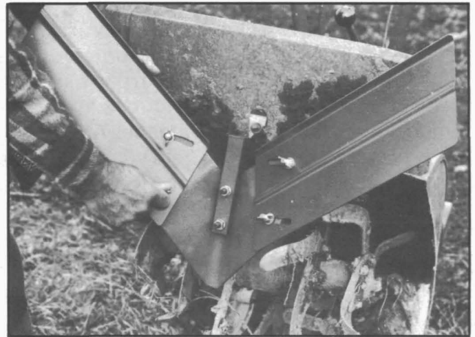
Hiller adjusts by hand—No tools needed.
