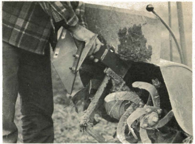
(Photo 6/48) Push "U" shaped bracket over depth adjustment bar. Install clinch pin.
