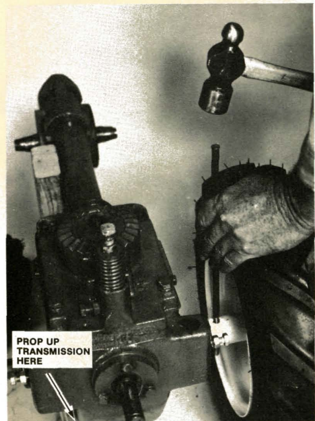
(Photo 8/129) Roll pin holds wheel on.
