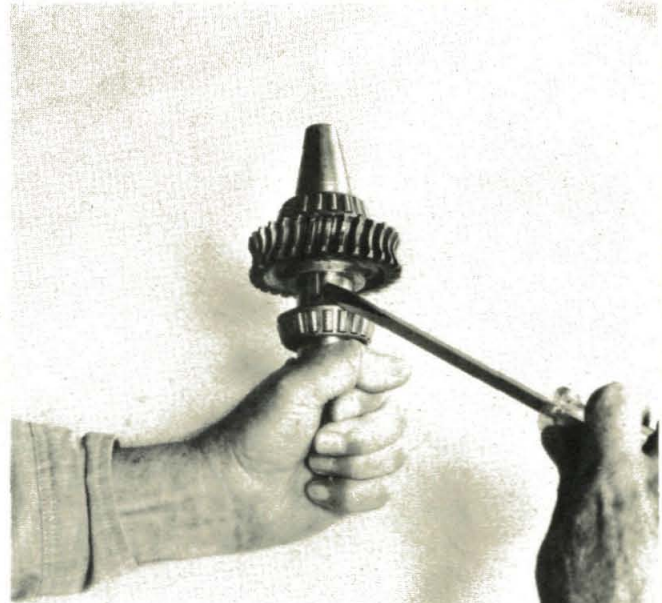
(Photo 8/15) Check key that drives bronze gear.
