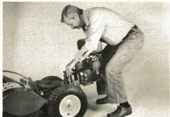
(Photo 8/107) Line up holes, put in bar.
