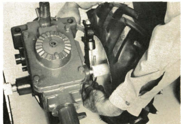
(Photo 8/3) Align holes with hex wrench.
