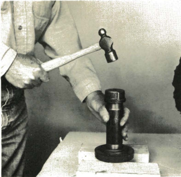
(Photo 8/12) Carefully tap seal out of cover.
