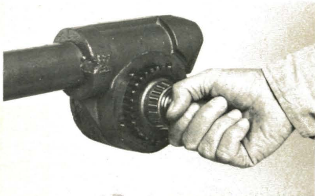
(Photo 8/18) Replace tiller shaft.
