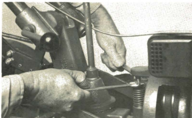
(Photo 7/29) Loosen locknut on adjustment bolt.
