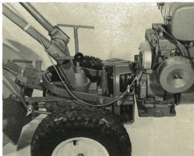
(Photo 4/27) Route cable outside of yoke.
