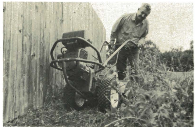
(Photo 6/27) Protects carburetor and engine from fences.
