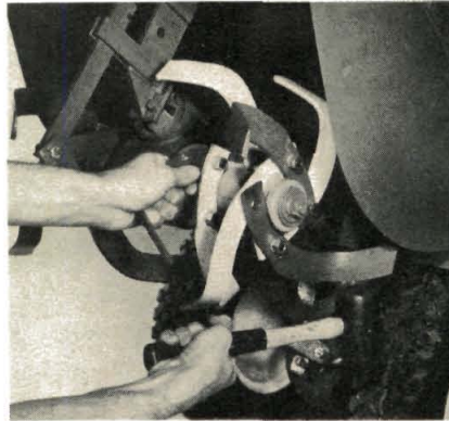
(Photo 8/64B) First, oil tight nuts. (Photo 8/64C) Tap tine to open. (Photo 8/64D) Repeat for inside.
