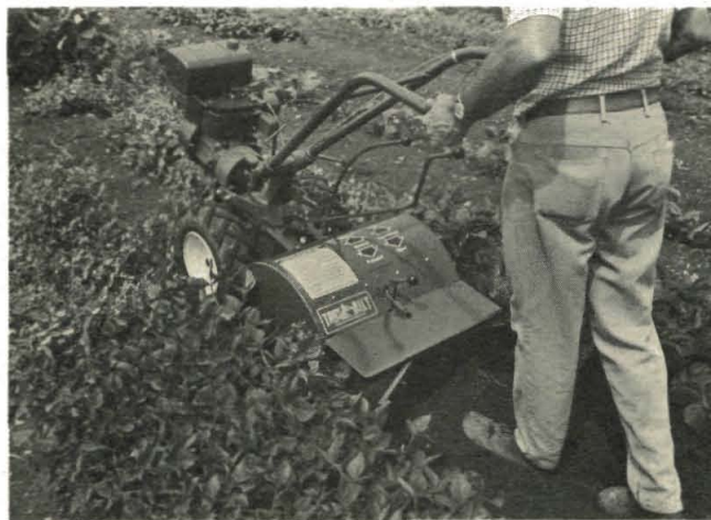
(Photo 6/41) Wings and tines work together. Tines chop up growth between rows.
