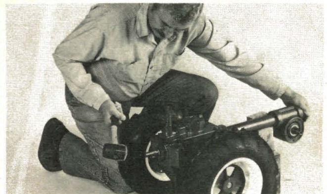
(Photo 8/39) Hold cap on, hit front of shaft.
