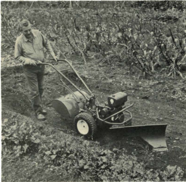
(Photo 6/16) Angle blade to one side to put soil where you want it.
