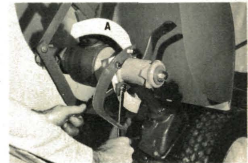
(Photo 8/57) Install an "A" gang
