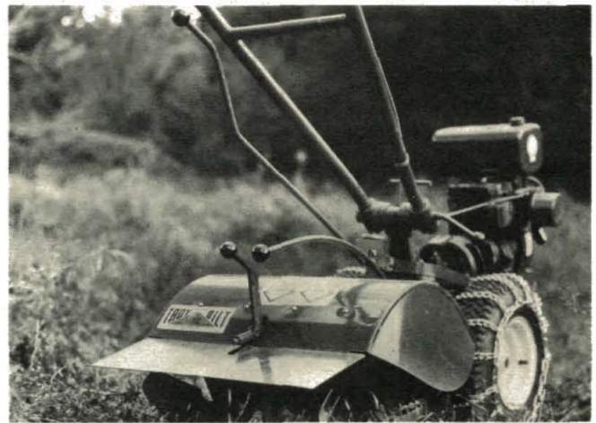
(Photo 6/44) In tackling tough sod, furrower can hold tiller back to allow tines more time to dig (use chains for traction)
