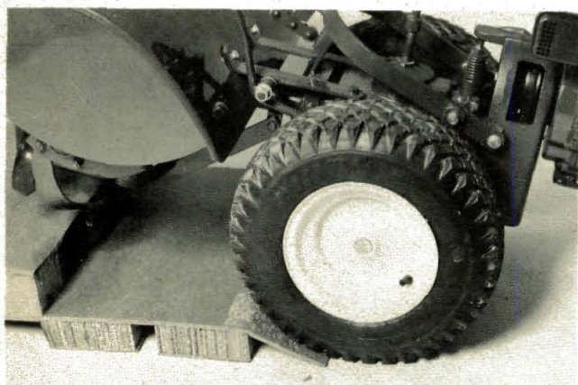
F. (Photo 1/3C) Grasp the Depth Regulator handle (the lowest lever in rear, center) and lift and roll the tiller off the container base. If the wheels won't turn, move the Wheel Speed Select Lever (on the right) a short distance to free the wheels.
