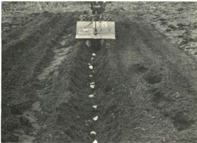
(Photo 6/34) The instant on-off Hiller/Furrower speeds and simplifies planting of potatoes. It makes furrows up to 8 inches deep.
