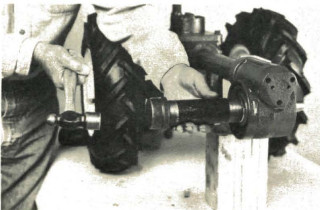
(Photo 8/21) Replacing seal with cover on.
