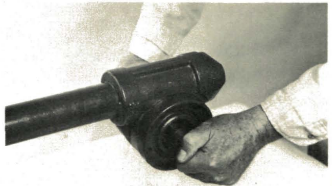
(Photo 8/22) Turn shaft forward and backward.
