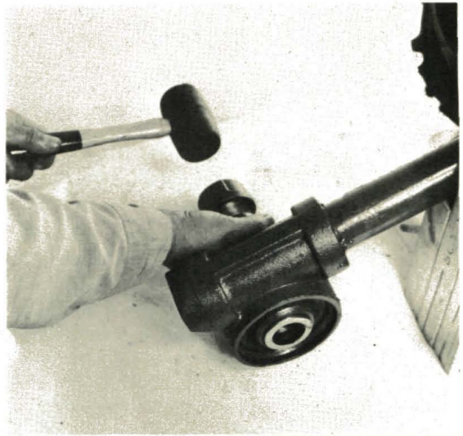
(Photo 8/14) Drive oil seal outward.
