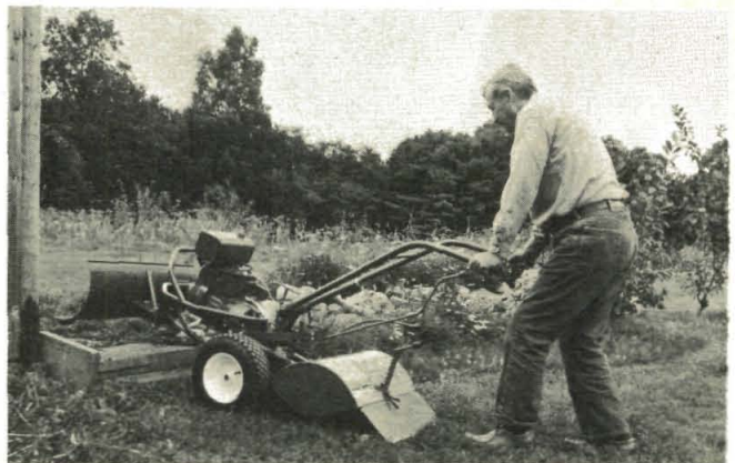
(Photo 6/23) Tine removal permits you to raise the front higher, and the blade banks easier.
