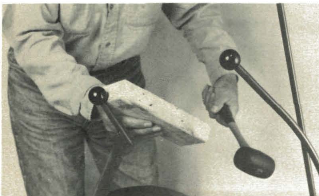
(Photo 8/42) Tap knob off, save tolerance ring.
