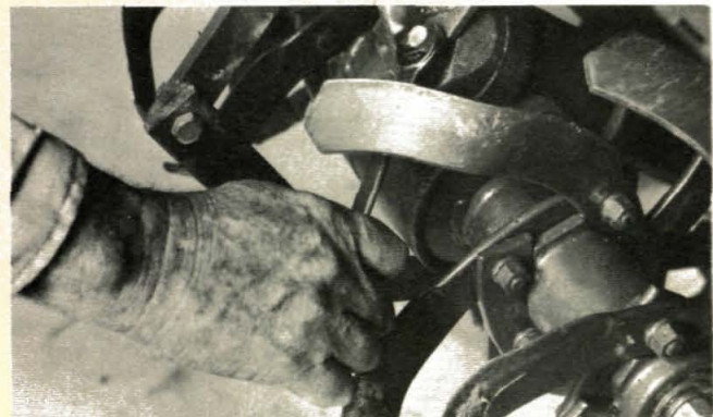
(Photo 8/122) Remove bracket bolts from end cap.
