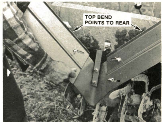
(Photo 6/50) Wings attach and adjust easily by hand. Wings go behind blade star washers up against wing.
