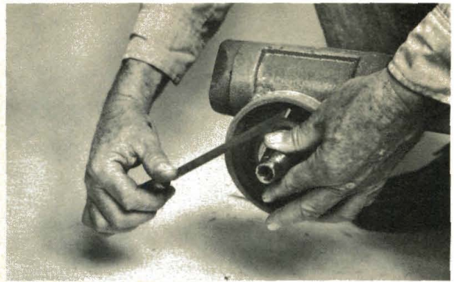
(Photo 8/138) Remove nicks and install tines.
