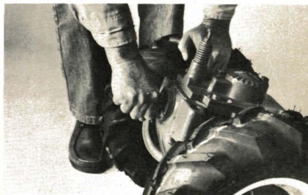
(Photo 8/30) Check for play in drive shaft.
