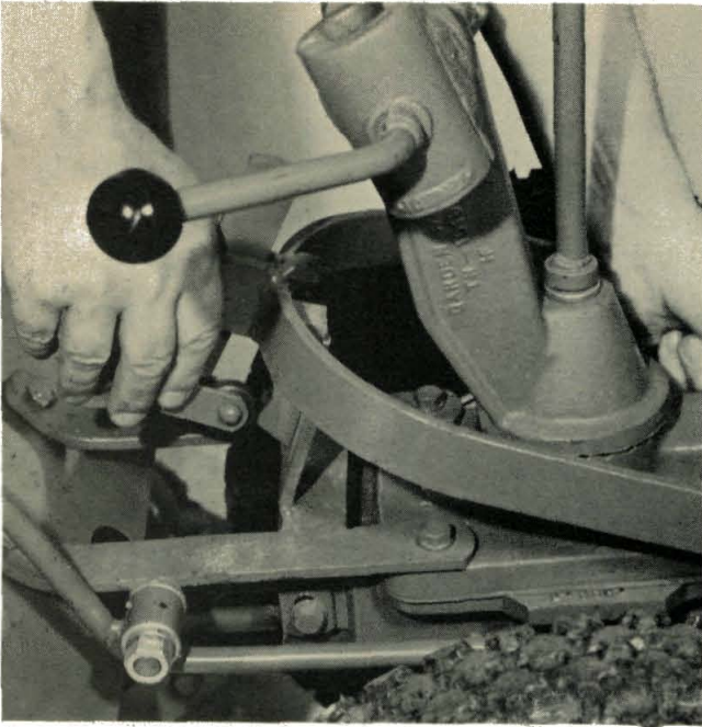
I. (Photo 1/6) Remove the wire holding the yoke. This will free up the yoke.
