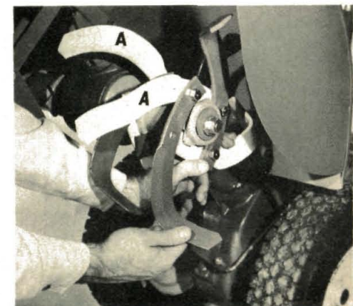
(Photo 8/58) Gang of tines marked with an "A" installed at positions 3 & 4. An "A" gang also goes at 2.
