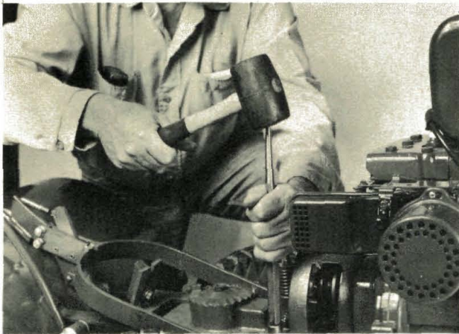
(Photo 8/109) Tap bars in place.
