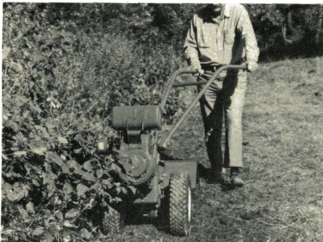
(Photo 2/10) To save your hands from being scratched by thorny bushes while tilling close to them, just move the handlebars to one side.
