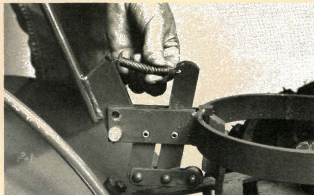
(Photo 8/148) Rehook lever and spring.
