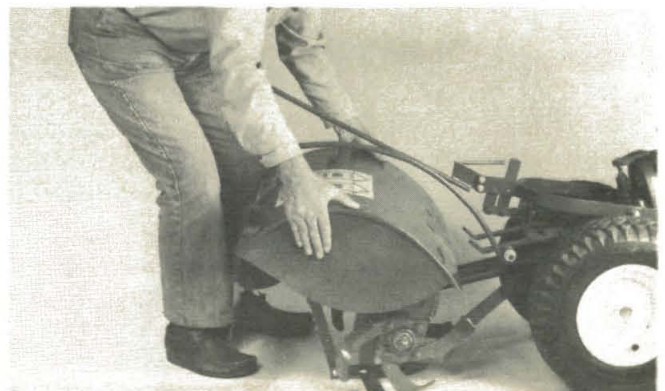
(Photo 8/43) Lift hood off.
