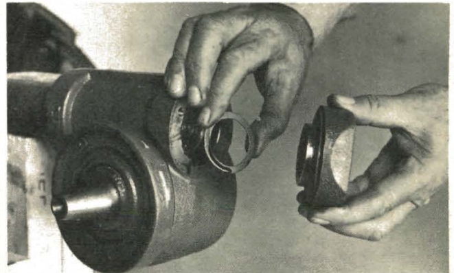
(Photo 8/37) Shims remove play in shaft.
