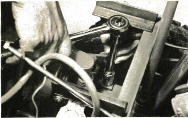
(Photo 8/134) Unbolt battery bracket.
