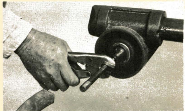
(Photo 8/128) Remove tine stud, watch threads.
