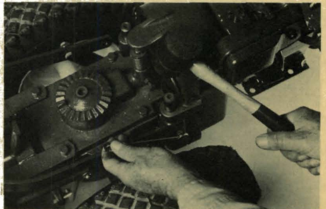
(Photo 8/147) Hold pressure on bolt and tap.
