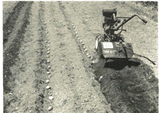
(Photo 6/35) When seed potatoes are in the ground, the labor saving Hiller wings will bury them. As potatoes grow, hill them as needed.
