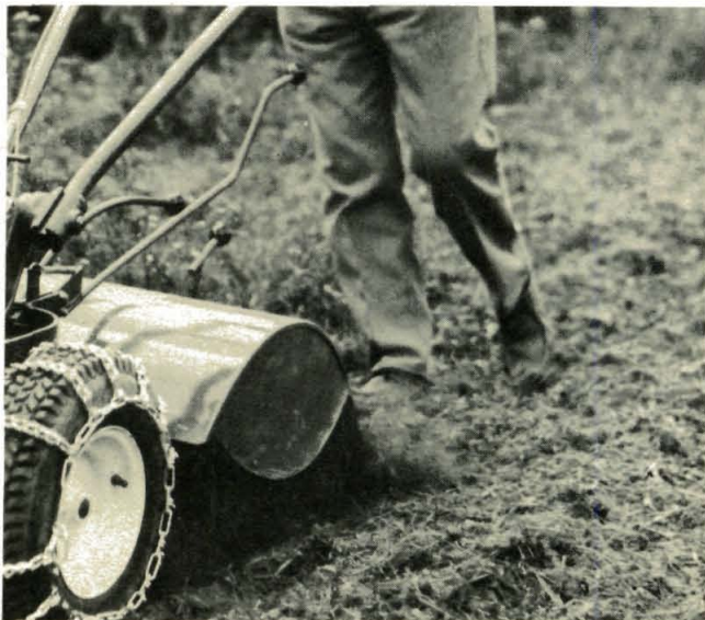
(Photo 2/17) Start shallow in new ground.
