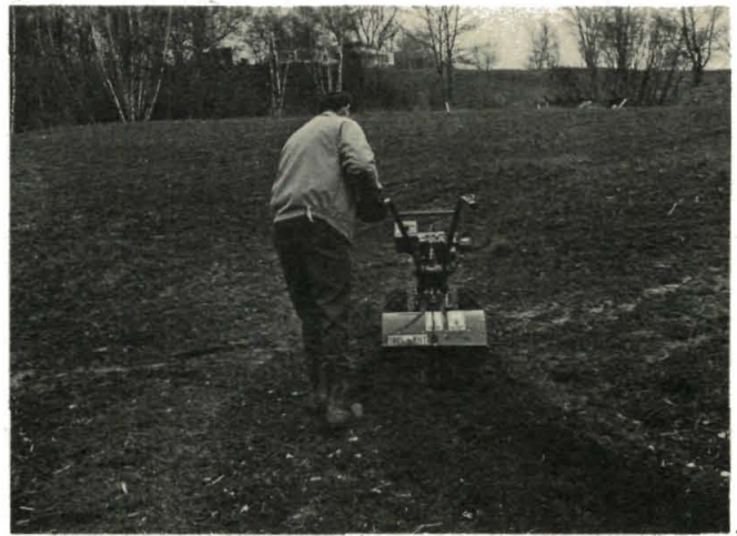
(Photo 6/43) Furrower can dig drainage ditch to dry up an area for early planting in springtime.
