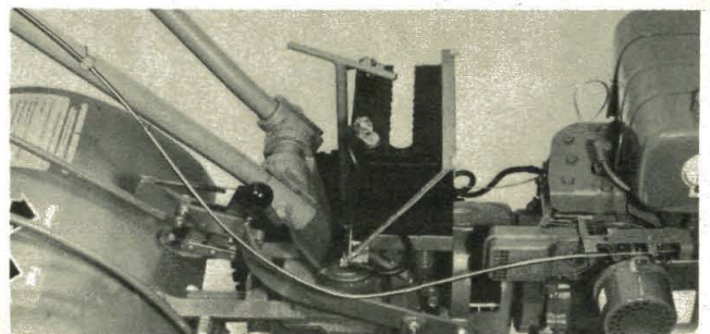
(Photo 4/10) Run throttle cable on electric start tillers down handlebars, as shown. Keep the throttle cable away from battery—6 HP electric start engine.
