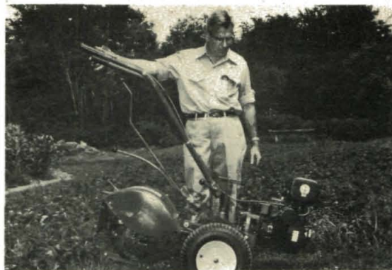
(Photo 5/21) The wheel axle serves as a pivot point to balance the weight of the tines in the rear against the weight of the engine up front.
