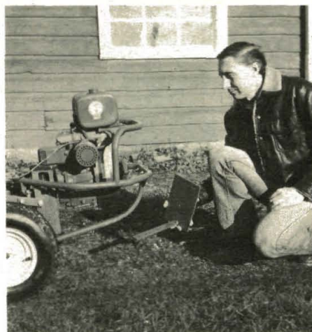
(Photo 6/32) It's easy to add the Dozer/Snow Blade to the Bumper—just add the brackets, the blade, and you're ready to go!
