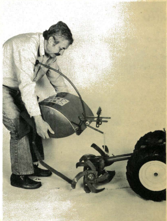
(Photo 8/126) Hood, lever & regulator come off.
