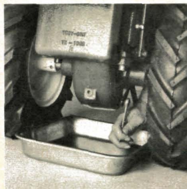
(Photo 8/113) Drain gear oil.
