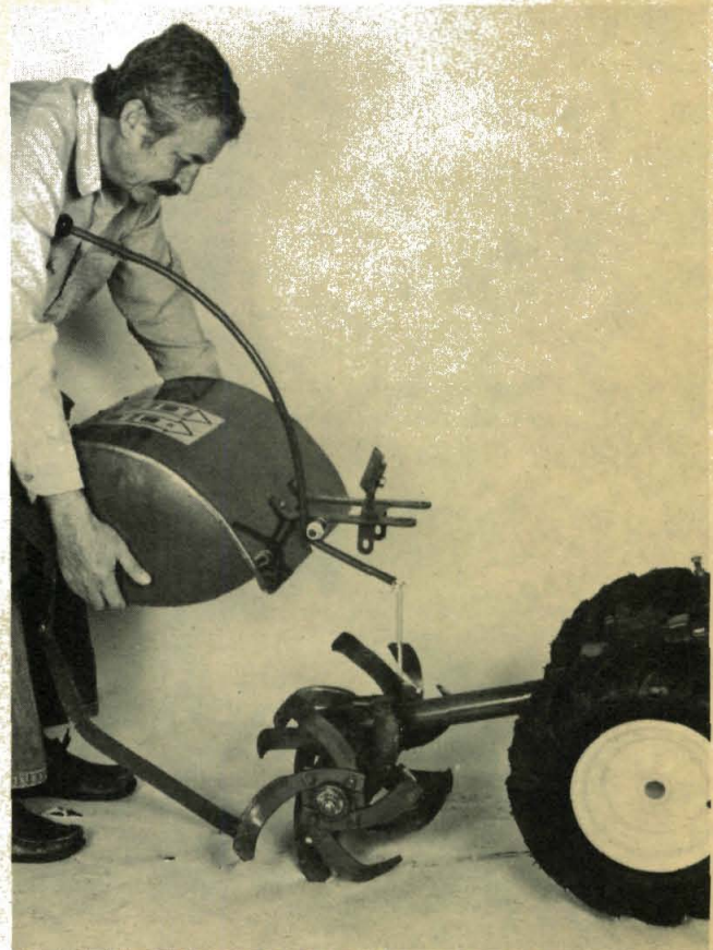
(Photo 8/140) Replace hood, lever and regulator
