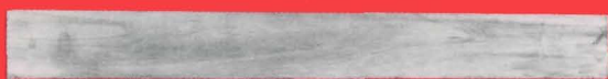
A short length of strong stick; 5/16" thick, about 1 3/4" wide, and about 12"-14" long.
