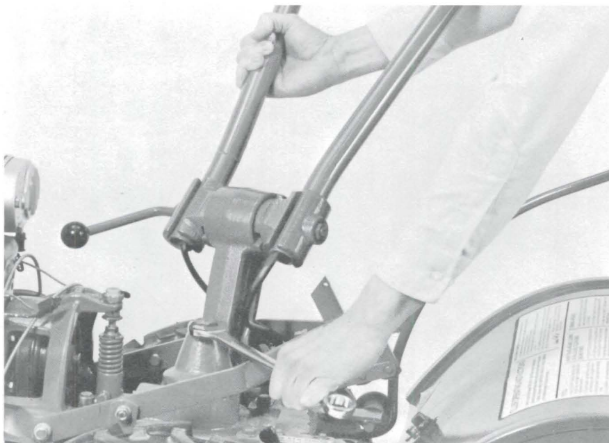
(Photo 11) Loosen bolt and swing handlebars to right side.
