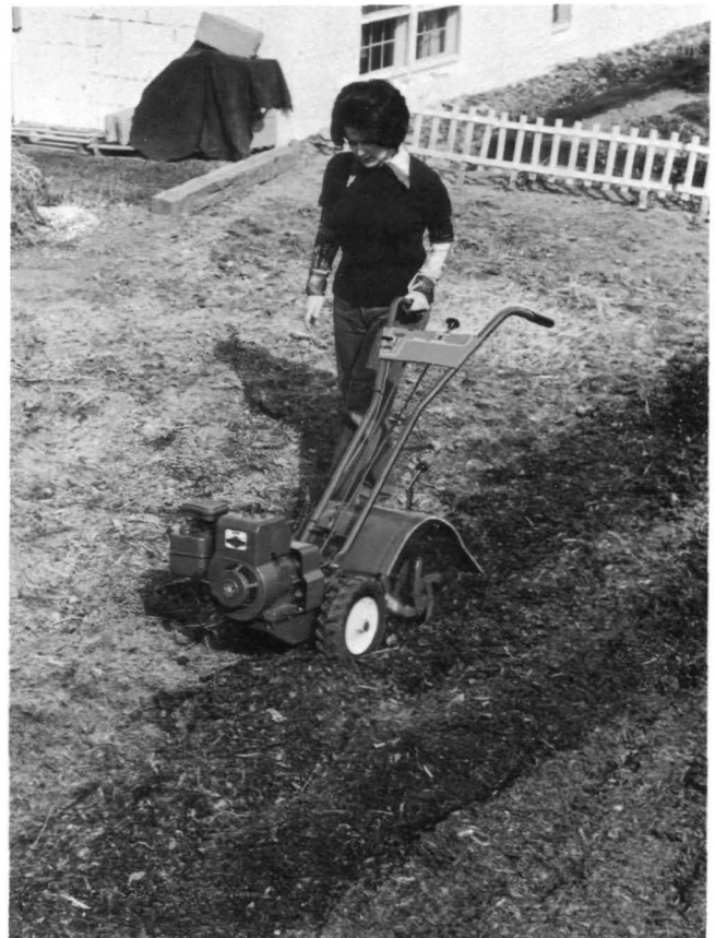
(Photo 5-27) Walk on untilled side, guiding tiller with one hand.
