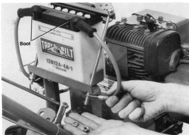
(Photo 1-32) Remove nut and lockwasher, put cable terminal on bolt, replace the hardware.
