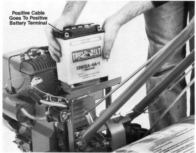
(Photo 1-29) Use two hands and position battery this way, positive (+) side to left rear of tiller.
