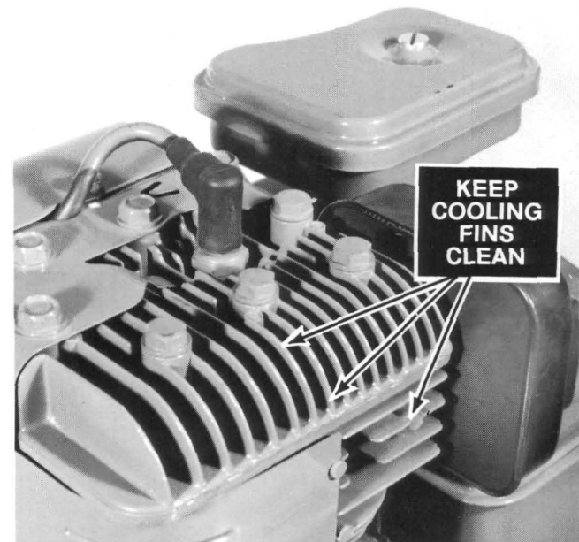
(Photo 6-7) Remove debris under blower housing.
