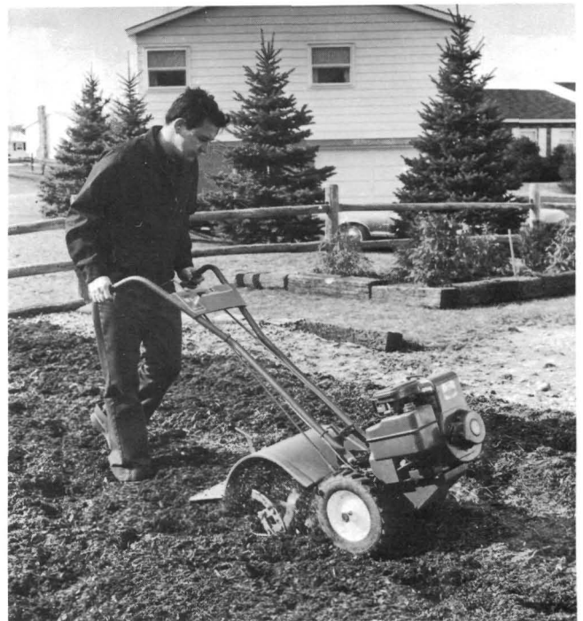
(Photo 2-15) In unworked soil with large hidden stones, use two hands until stones are cleaned out.
