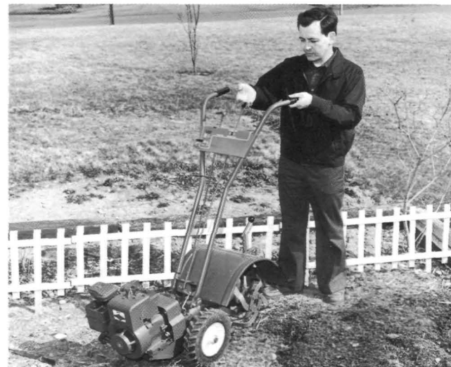
(Photo 5-22) Use reverse to turn in close quarters: keep handlebars up; balance tiller weight; and PULL out on the Forward/Reverse Lever to back up briefly. This allows you to complete your turn in a small area.
