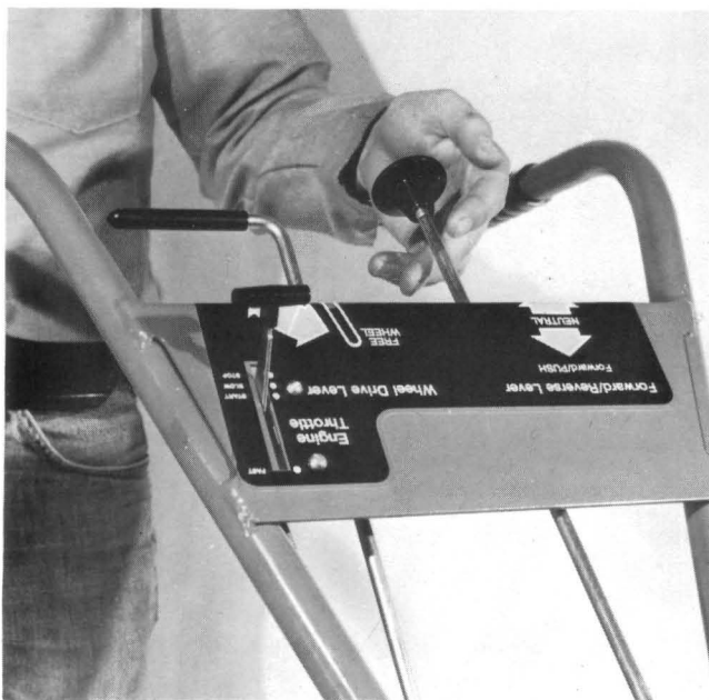
(Photo 2-9) Release lever to stop Reverse.
