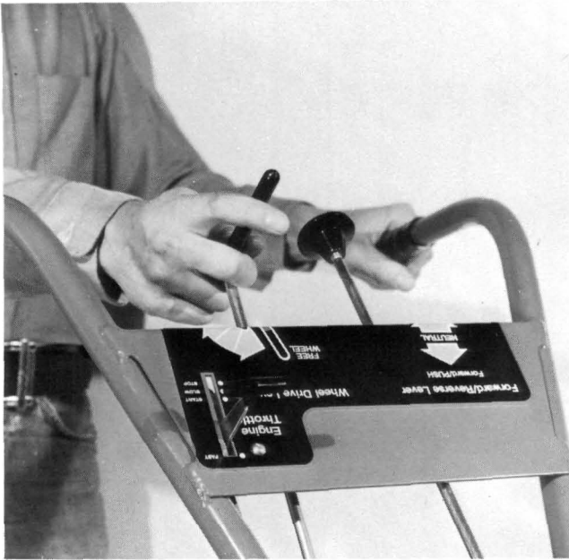
(Photo 1-23) Point lever towards Free Wheel on control panel label.
