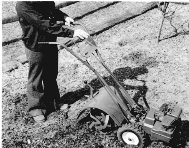
(Photo 5-14) When you have put the Wheel Drive Lever in DRIVE, line up with your row and PUSH for Forward.
