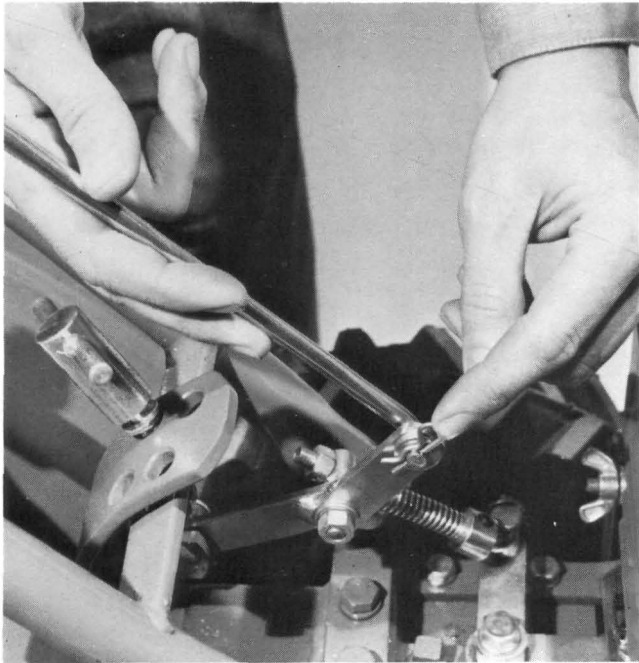
(Photo 1-20) Insert hitch pin.
