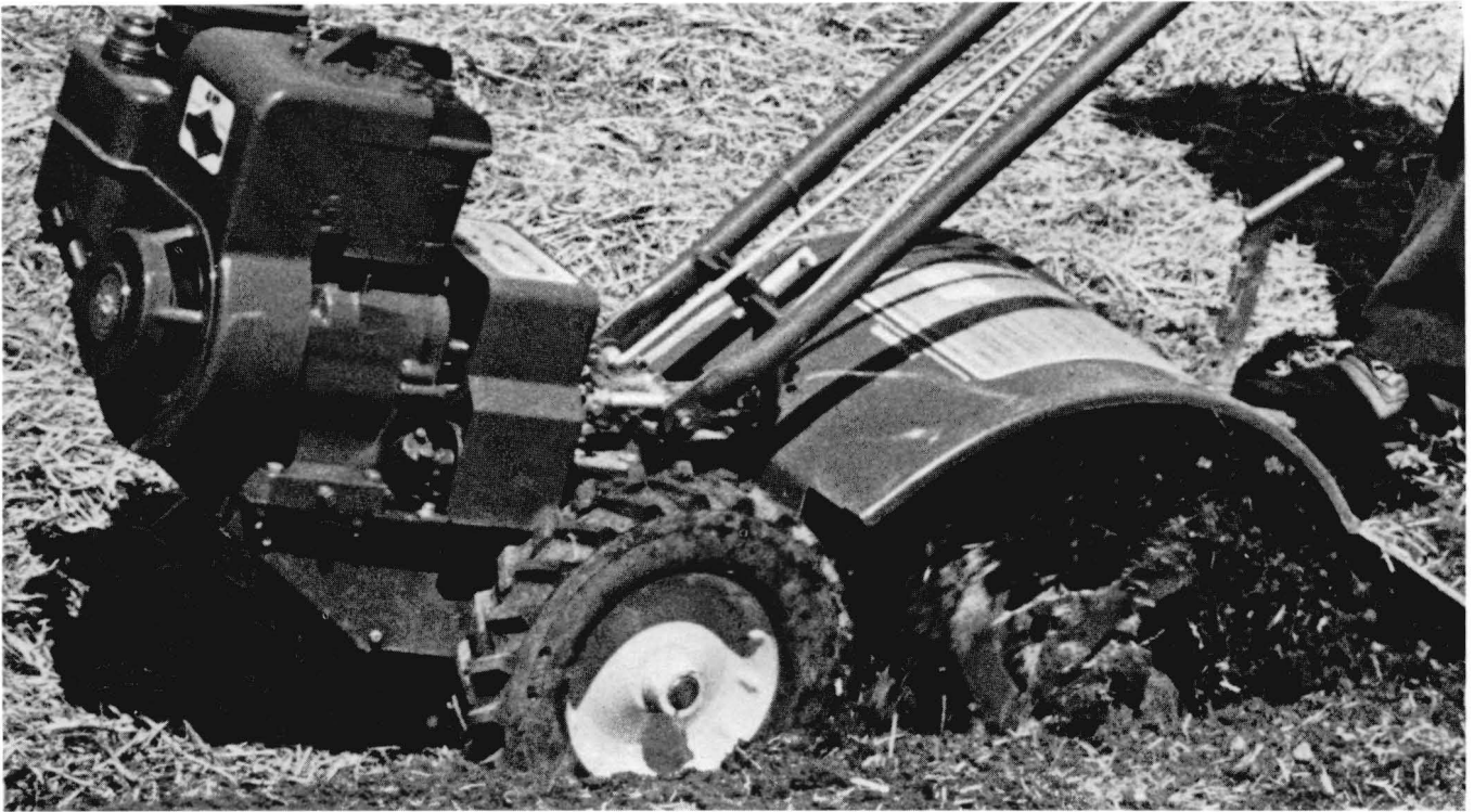
(Photo 5-1) Tilling the Troy-Bilt way with tines in the rear.
