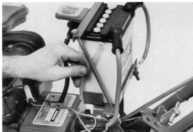
(Photo 1-33) Vent tube first goes down through rigid tube, then up onto vent fitting. For safety, make sure it's not kinked.
