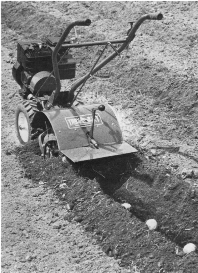
(Photo 5-44) Furrow to plant potatoes. Use the Hiller wings to cover them up and later to hill the potato plants.
