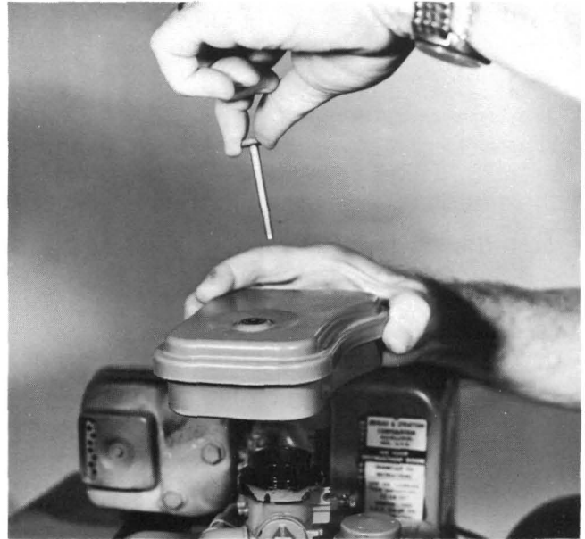
(Photo 6-5) Air cleaner removal
