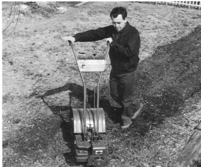
(Photo 5-18) Balance the weight of the engine in front with the tines in the rear. Use your arms to push the handlebars sideways to move the tiller in the direction of your turn.
