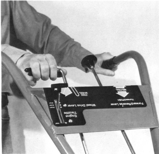
(Photo 2-3) Wheel Drive Lever in DRIVE.
