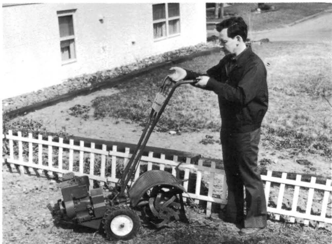
(Photo 5-10) For reverse, lift handlebars and pull Forward/Reverse Lever out.
