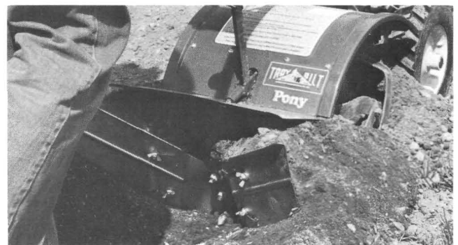
(Photo 5-42) Furrower Blade with Hiller Wings lets you make rows, trenches, ditches.
