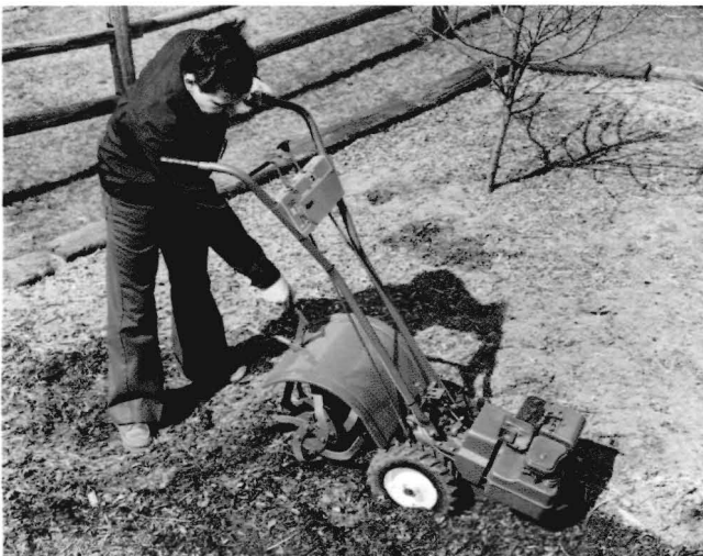
(Photo 5-12) Before tilling, set the depth regulator — shown in the photo.
