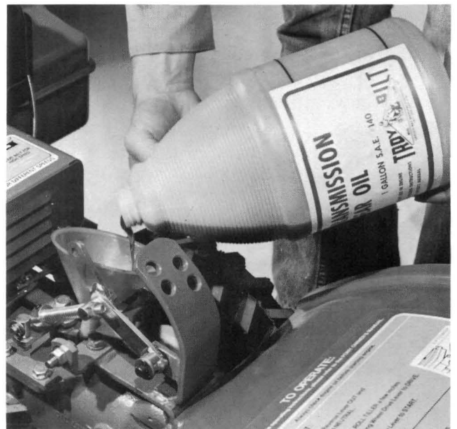
(Photo 1-5) Add gear oil if necessary.
