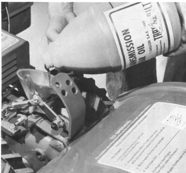
(Photo 6-3) If you add gear oil, keep tines off floor
