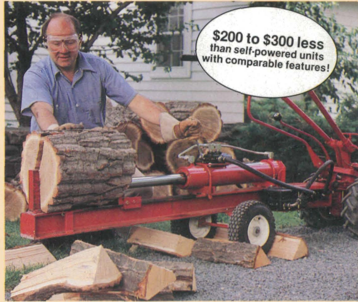
Drive the PTO Hydraulic LOG SPLITTER right up to your woodpile...split as much as a full cord an hour!
