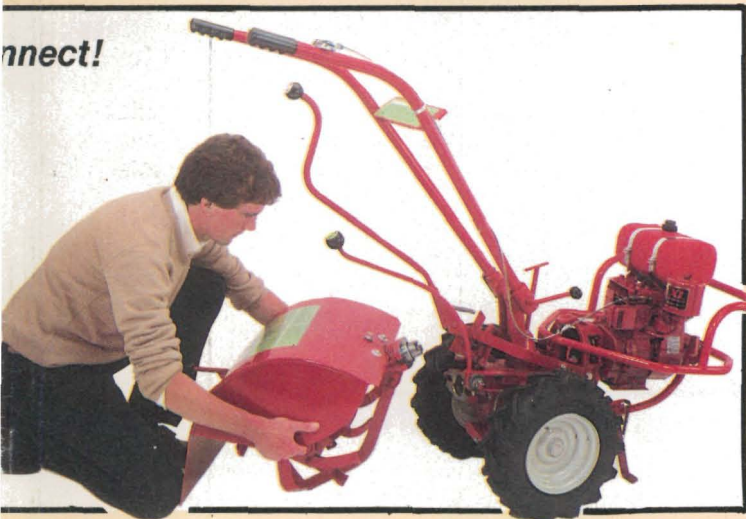
Using the super-sturdy Troy-Bilt TOW HITCH, the PTO Horse model can also pull lawn rollers, sprayers and other standard pull-behind equipment!
