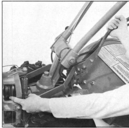
Photo 4-15: With Wheels/Tines/PTO Drive Lever held UP in REVERSE, move belt on engine (upper) pulley over into its rear groove.
