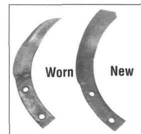
Photo 5-30: Check for tine wear every 30 operating hours.
