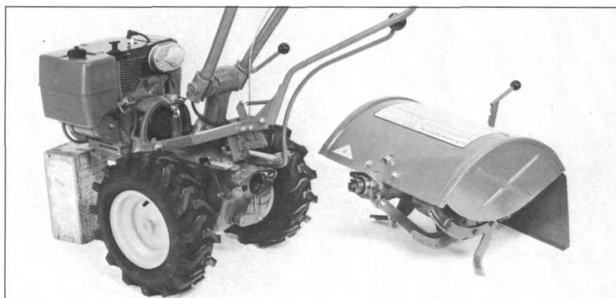
Photo 4-36: The PTO Power Unit with the tine attachment removed.
