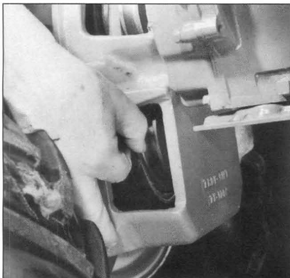
Photo 5-17: First move belt off the lower pulley.
