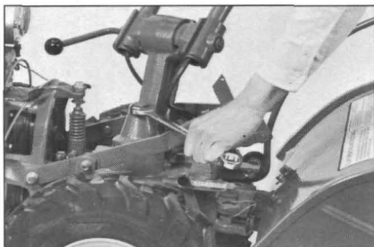
Photo 2-8. Loosen the large bolt securing the handlebar base. Swing handlebars to right side.
