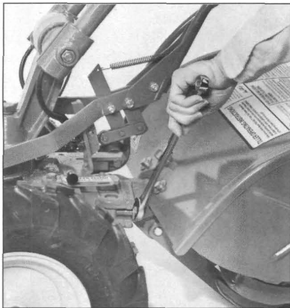
Photo 4-44: Tighten both swing-bolts very securely with a long 3/4" wrench. Tighten them to between 70-to-80 ft. lbs.
