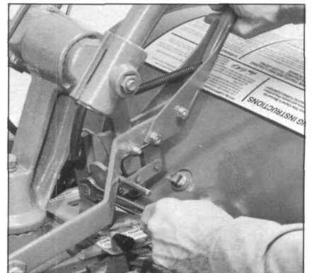
Photo 5-16: Hold Drive Lever while loosening bolt. Push lever down to tighten belt; pull up to loosen belt.
