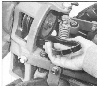
Photo 5-20: Shift into FORWARD and remove the belt.
