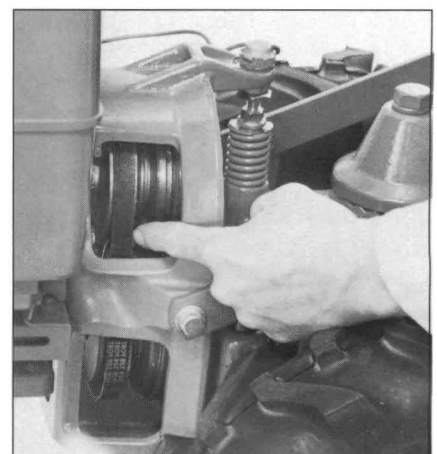
Photo 4-14: Move belt on the engine pulley into the forward groove.
