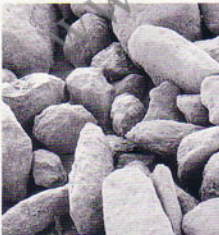
Electron Microscope photos of soil show loose grains in a sandy soil (left). No wonder water pours through! The same soil (right) with organic matter, binds particles together, so soil retains moisture, nutrients.
