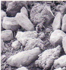
Electron Microscope photos of soil show loose grains in a sandy soil (left). No wonder water pours through! The same soil (right) with organic matter, binds particles together, so soil retains moisture, nutrients.
