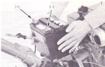
(Photo 33) Battery posts face to rear of tiller.
