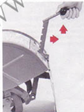
(Photo 20) Pull Depth Regulator Lever back and then up.
