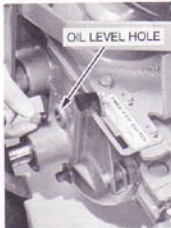
(Photo 21) Gear oil should seep from oil level check hole.
