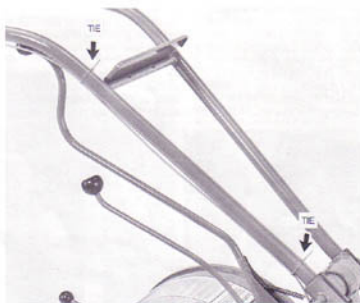
(Photo 28) Secure cable with plastic ties.
