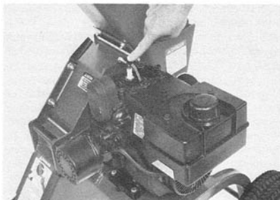
(Photo 3-10) Engine Shut-Off Tab. Push against spark plug to stop the engine.
