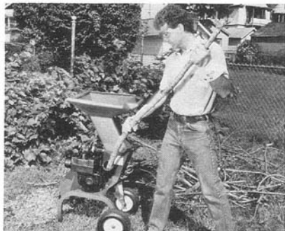
(Photo 4-4) If engine speed starts to slow, reduce feed pressure and let engine speed build up.
