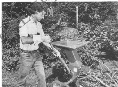
(Photo 4-3) Hold branches firmly; feed in smoothly.
