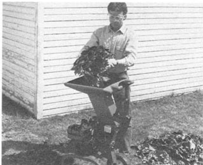
(Photo 4-6) Feed materials in steadily and slowly, but don't overload the shredder. Your Leaf Tamper can hang conveniently on the shredder handle, ready for use.
