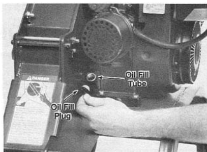
(Photo 2-3) Turn Oil Fill Plug counterclockwise to remove it from the Oil Fill Tube. If tight, use a screwdriver blade as a lever between the two posts.
