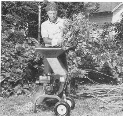
(Photo 4-5) When using the Shredder, stand 1-to-2 feet away from the top-loading hopper and release materials into it.
