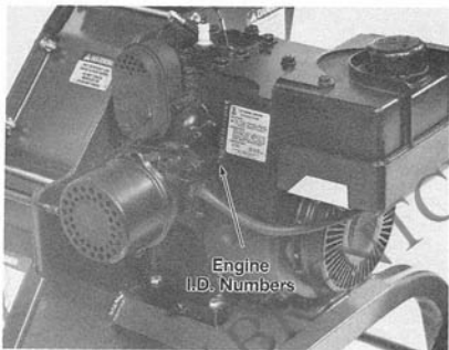
(Photo 5-1) Location of Tecumseh engine I.D. numbers.
