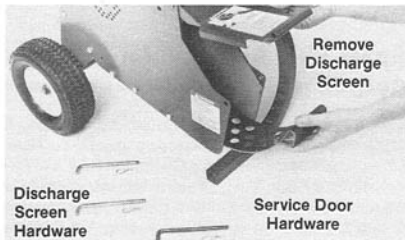
(Photo 5-8) Remove the Discharge Screen. First, pull out the two hair pin clips and slide out the two rods securing the discharge screen. While holding up the service door slide the screen out and put it aside with its hardware. Note how the screen ends are different — during reassembly, the end that's bent back the most goes in first.
