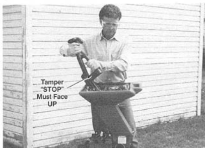
(Photo 4-7) Use your Leaf Tamper to push loose materials into the shredder-chamber. Position the Tamper so the "stop" faces UP as shown in the photo. The "stop" prevents the Tamper from going too far in.
