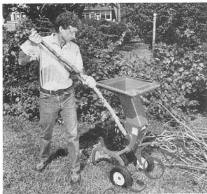
(Photo 4-2) Feed material into chipper at proper angle, and rotate branches. Do not overload the chipper.
