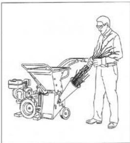
Photo 4-10: Using the chipper for small branches.
