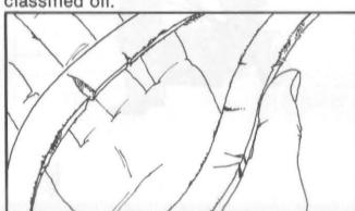
CHECK DRIVE BELT(S) for proper tension and wear. Replace belt when overstretched, cracked or severely worn.
