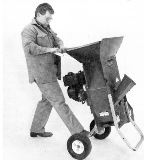
(Photo 4-1) To move your Chipper/Shredder, plant one foot on the axle, tilt equipment back with both hands until "balance point" is reached, then push or pull your equipment to a work area. Engine must be OFF.
