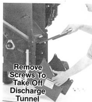
(Photo 5-18) To take off discharge tunnel for more working room, remove three screws from frame on chipper side, then do the same on the engine side.
