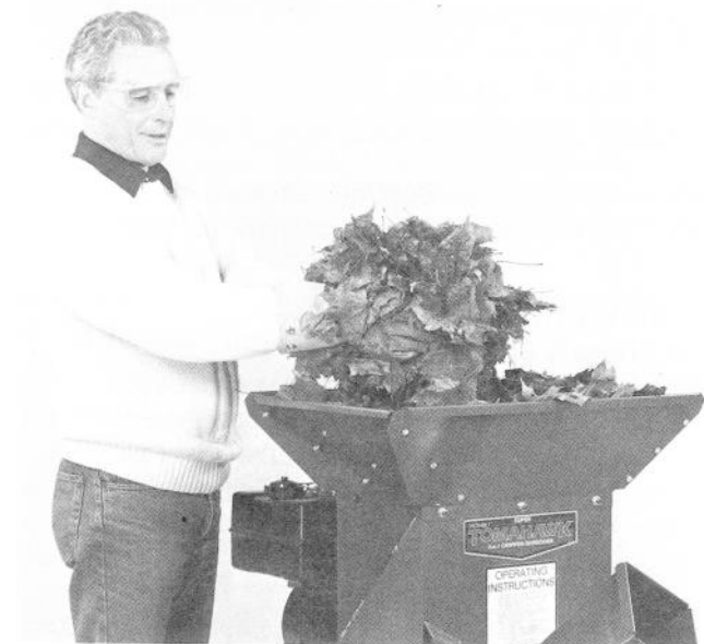
(Photo 4-5) When using the Shredder, stand 1-to-2 feet away from the top-loading hopper and release materials into it from any position within the "Operation Zone".
