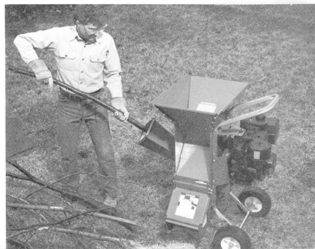
(Photo 4-4) If engine speed starts to slow, reduce feed pressure and let engine speed build up.
