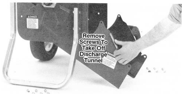
(Photo 5-22) Take off three screws on both sides of the shredder in order to remove the discharge tunnel. This gives you a lot more room to maneuver.
