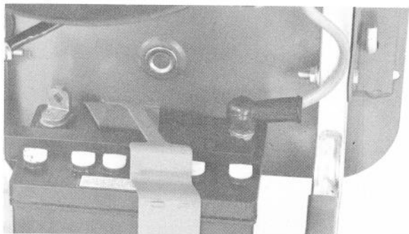
(Photo 2-19) Slide the rubber boot over the battery post and the end of the positive cable (8HP system shown).
