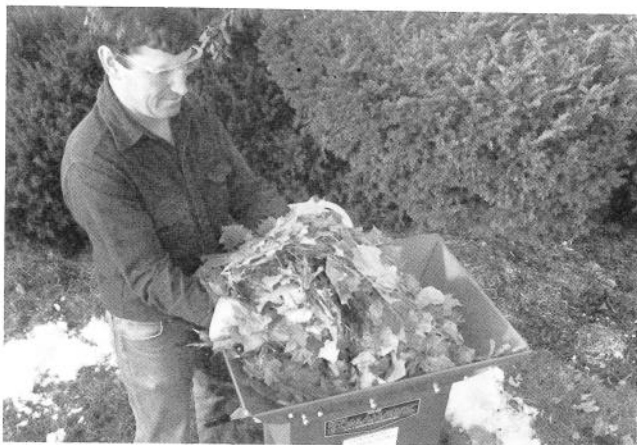
(Photo 4-6) Feed materials in steadily, but don't overload the shredder.
