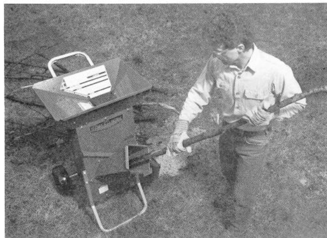
(Photo 4-3) Hold branches firmly; feed in smoothly.
