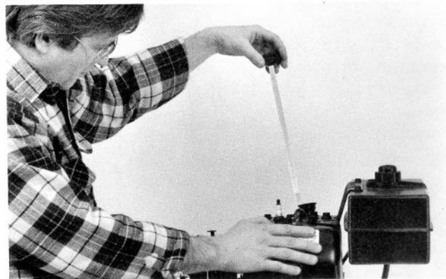
(Photo 2-6) On 5 HP Tecumseh engines, remove oil dipstick from oil fill tube, then add 19 ounces of motor oil using a clean funnel. Fill to "Full" mark on the dipstick. Do not overfill!
