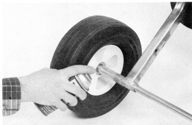
(Photo 5-7) The wheels and axle spacers should also be lubricated regularly.
