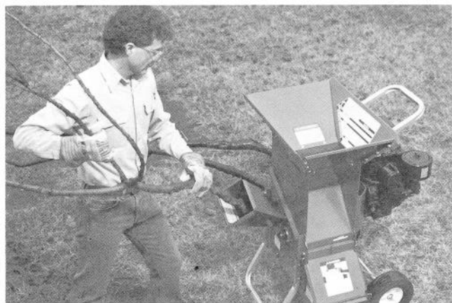
(Photo 4-2) Feed material into chipper at proper angle, and rotate branch. Do not overload the chipper.
