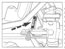
The Horse Tiller Model & Serial Number is on top of the transmission. Check your numbers against the one listed at left. The first five digits are the Model Number. The digits after the Model Number make up the Serial Number.
